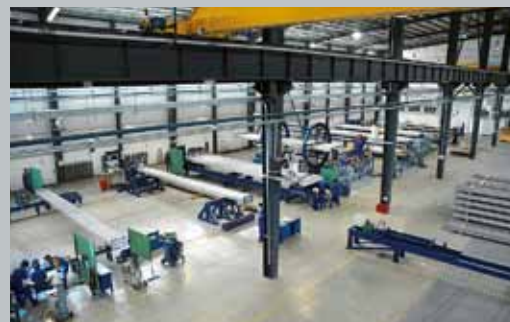
Highly standardized manufacturing site for Alex air-cooled condenser bundles
